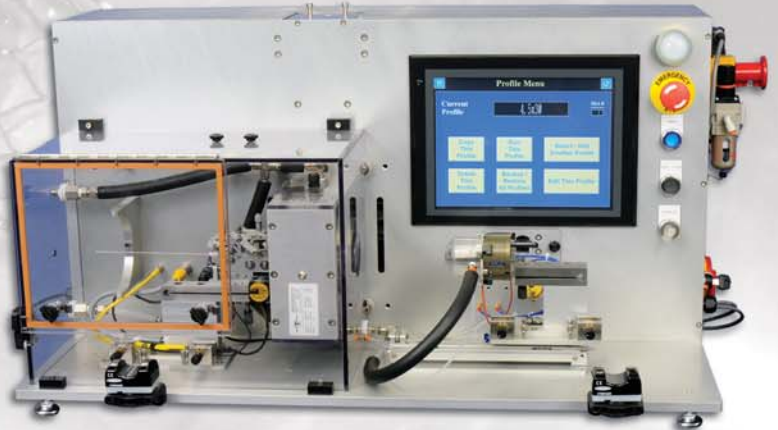
Automated, PLC Controlled Configuration
